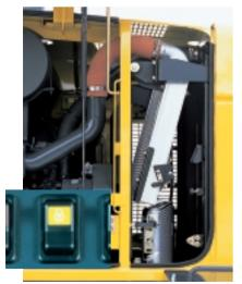
If the machine is operating in adverse conditions, the operator can reverse the hydraulic cooling fan from inside the cab by turning on a switch on the control panel. The coolers can also swing out for easy cleaning.
